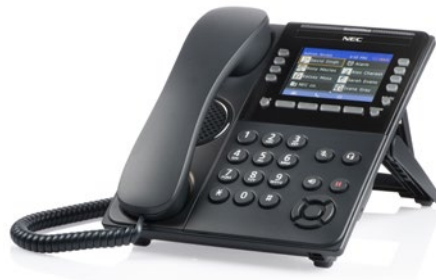
DT930S Self-labeling with color display
